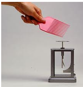
Fig 8.15 Deflected leaves of an electroscope
