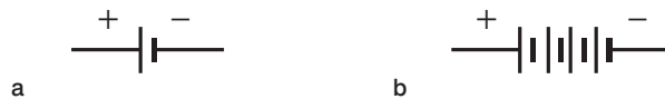
Figure 3.24 a) The symbol for a cell; b) a battery of four cells.
