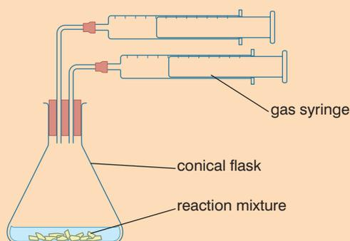
**Figure 3.18** Apparatus set-up
