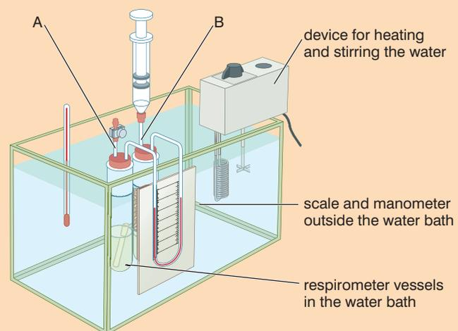
Figure 5.20 Using the respirometer in a water bath
