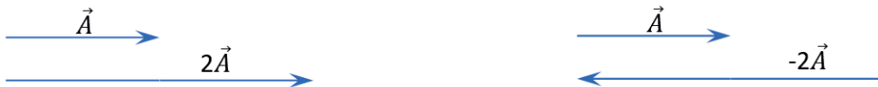
Figure 2.26 (a) \vec{A} and 2\vec{A} are parallel (b) \vec{A} and -2\vec{A} are antiparallel
